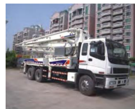
120M H CONCRETE PUMP
